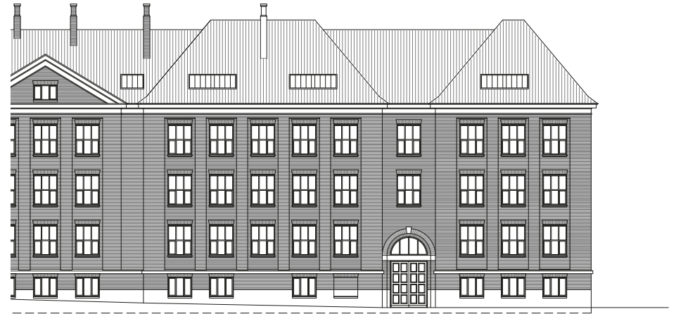
Fig. 28a. Existing terrain and floor level (dashed line).
