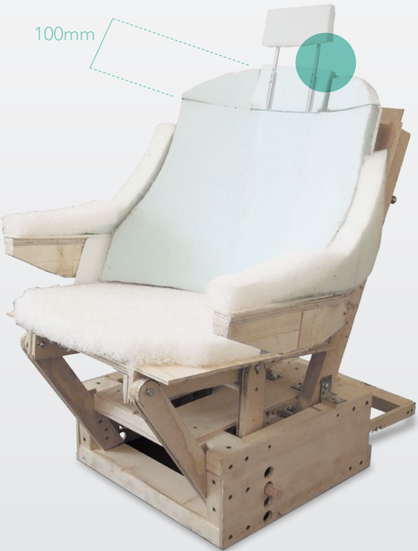
Ill. 103.d 100mm of back height added to the mock up. The slide system was also tested.
