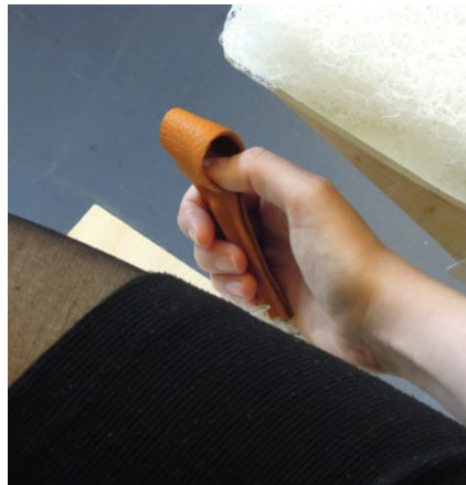
Ill 114.d: Handle three Leather is folded around the a round metal profile.
