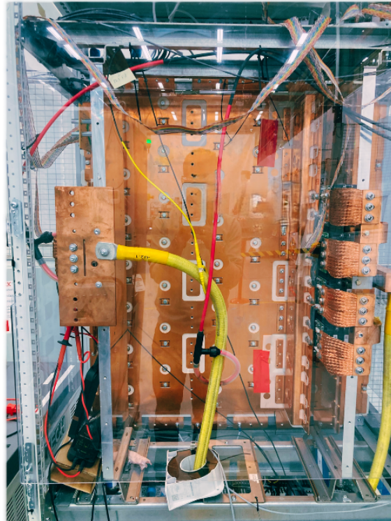
Figure 7.8: Double Pulse Setup with new busbar
