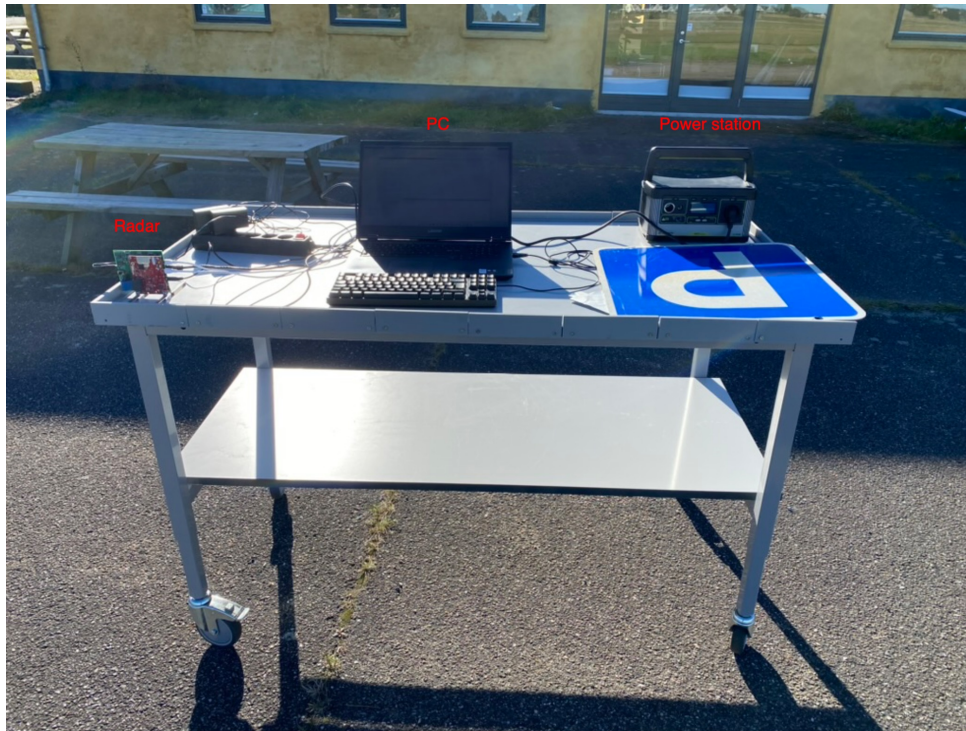
Figure B.1: Setup for the radar angle test (first view).
