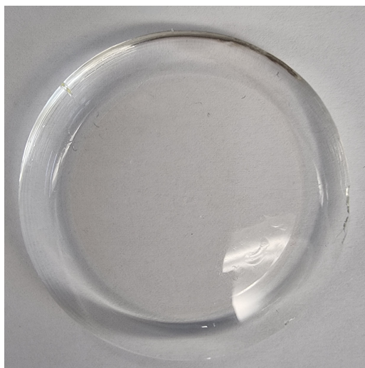
TPI ratio: 0.5 without catalyst TPI0.5-PEG200-N-TEOS30-S-a
