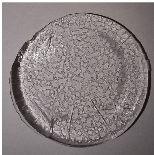
TPI ratio: 3.0 With Catalyst TPI3.0-PEG200-C-TEOS30-S-a
