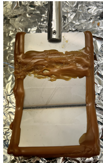
Figure 33: Three-electrode setup with bent and purpose of experimental process development testing Figure 34: 304SS welded coupon setup for CPP with the purpose of experimental process development testing
