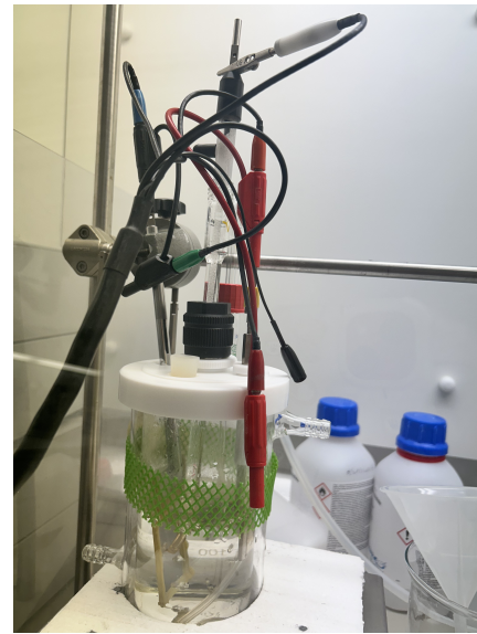
Figure 26: Jacketed Corrosion Cell Used for Testing 304 SS Coupons
