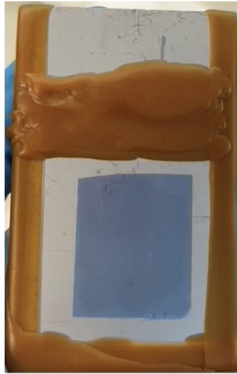
Figure 27: Example of a 304 SS Coupon that was passivated with the taped area sealed from the nitric acid passivation sol., and later waxed.
