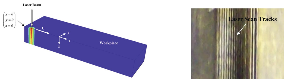
Figure 6: Diagram of laser heating process, in Figure 7: Laser generated scanning marking/tinting indicating localized heating, and its coordinate system [17].
