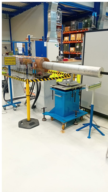
Figure 3.10. Whole translation system with the tube in the aperture of the magnet and the sliding system on the right side of the image.
