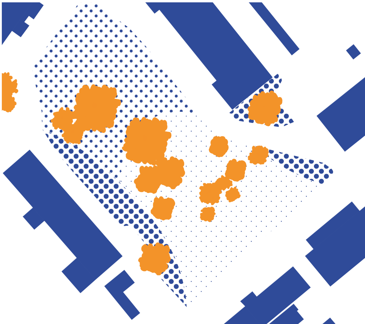
Illu. 36. Shadow diagram, the intensity of the hatch, determines the amount of shadow, 1:500
