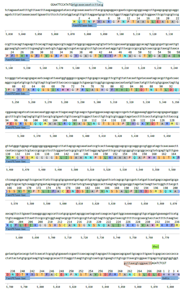
Figure 6.10. Sequence of (A) LCC ICC -bac in pET32a+ and (B) FastPETase-bac in pET28a+. The sequence was codon optimized for B. subtilis and then forwarded to Gene Universal to be synthesized and cloned into the vector pET32a+ or pET28a+, respectively. The primers used for PCR amplification of the genes are highlighted. Visualisation and Annotation were generated with Benchling.
