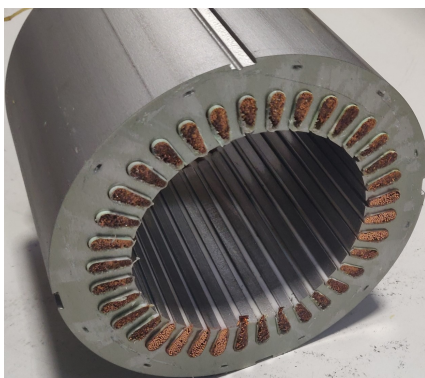
Figure 7.1: Stator after cutting
