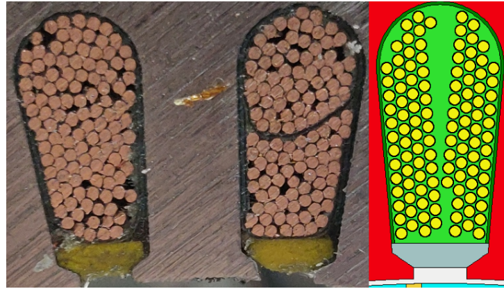
Figure 8.4: Difference between slot cross-section of UMP-3C3-210-25-4 in reality and in MotorCAD
