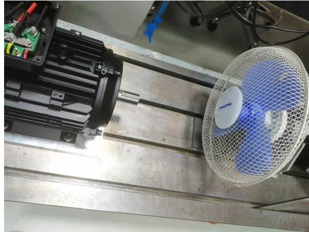
Figure F.2: External fan for cooling of FAB112M
