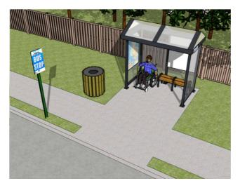
Figure 21. Representation of a wheelchair-friendly bus stop design. National Aging and Disability
