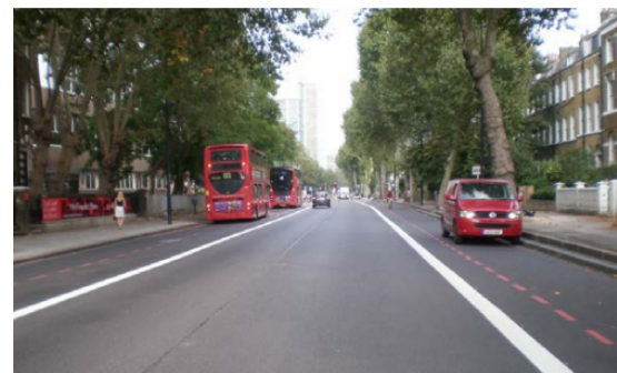
Figure 4.16. Example of narrow traffic lanes to encourages slower driving (Transport For London, n.d.).
