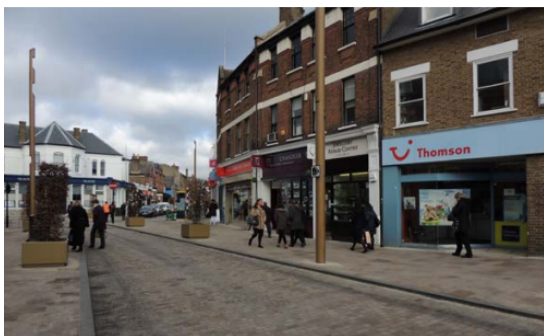
Figure 4.11. Example of a narrow carriageway to make people drive slow (Transport For London, n.d.).
