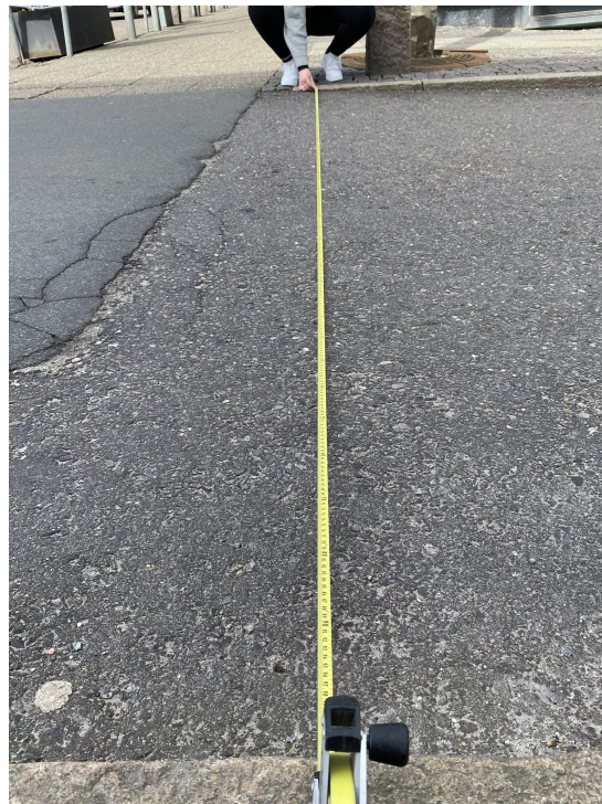
Figure 2.6. Picture from Holsteinsgade where the width of the traffic lane is measured.
