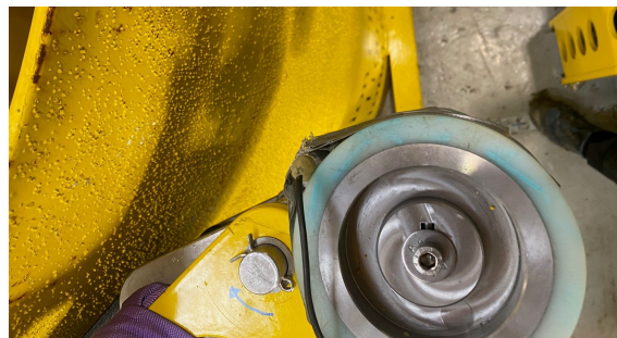
Figure 9.1: Location of load cell attached to wheel before being pressed against the member
