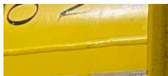
Figure 3.6: Welding seam across the offshore test member at SubC Partners.
