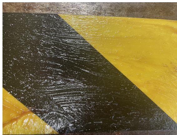
Figure A.6: Greasy surface when used SKF Bearing grease.
