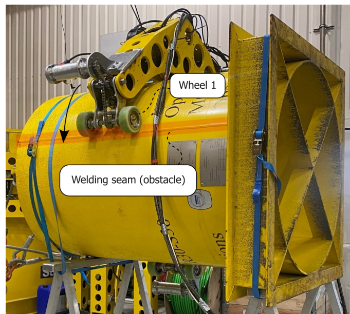
Figure 12.1: Physical test setup used for testing controller performance with varying velocity references and welding seam used as obstacle for the crawler to overcome
