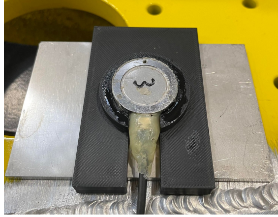
Figure 9.5: Updated casing for the load cell
