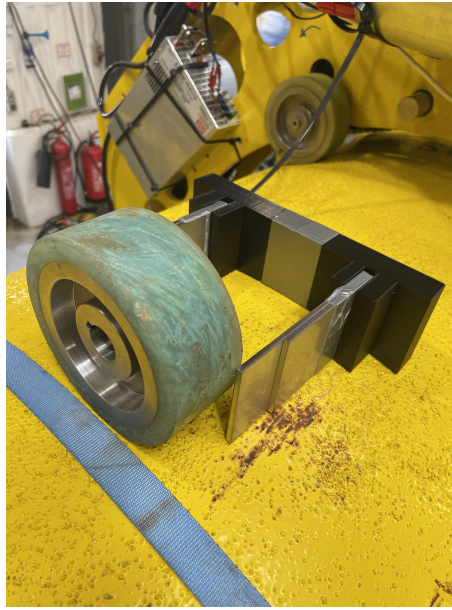
Figure A.2: 3D printed solution for testing of the rough surface of the offshore member.
