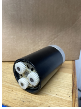
(a) A low-speed gearwheel connected to the shaft of the Maxon motor and gearbox, inside the waterproof casing.
