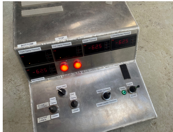
Figure 3.2: Manual pilot control panel for the offshore Crawler
