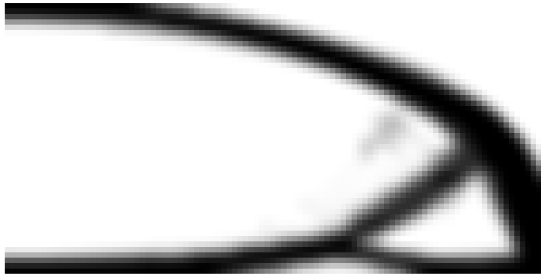
Figure 6.7. Design after 20 iterations, remaining volume is 25%.
