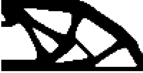
Figure 6.12. Compliance minimized MBB without continuation. Compliance is 1.598 Nm. Converged in 50 iterations.
