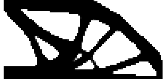
Figure 6.13. Compliance minimized MBB with continuation. Compliance is 1.583 Nm. Converged in 104 iterations.
