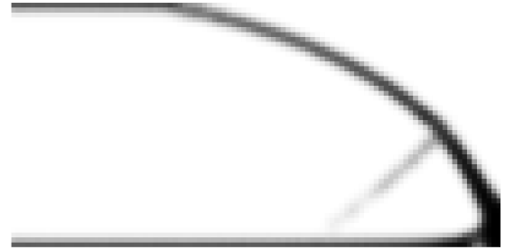
Figure 6.8. Design after 200 iterations, remaining volume is 7.4%.
