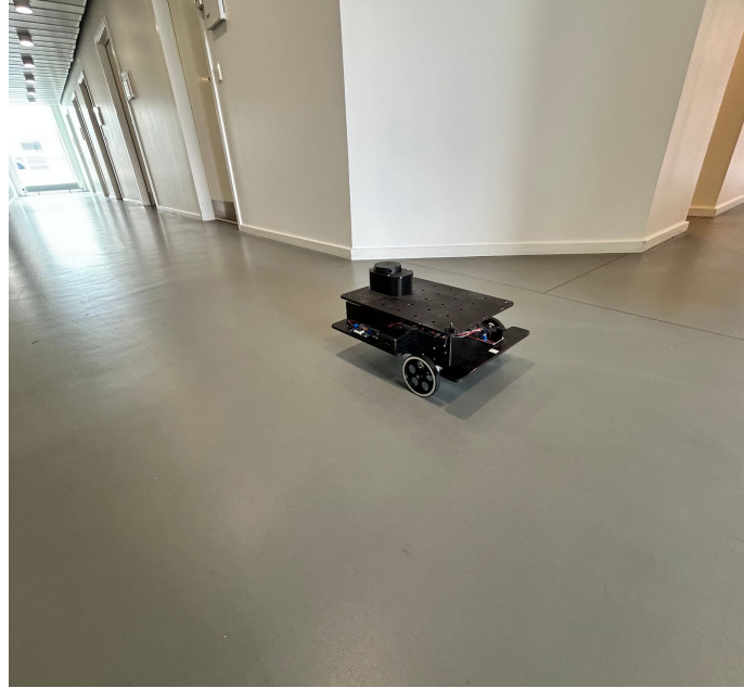
Fig. 38: Physical AMR with original wheels providing slippage
