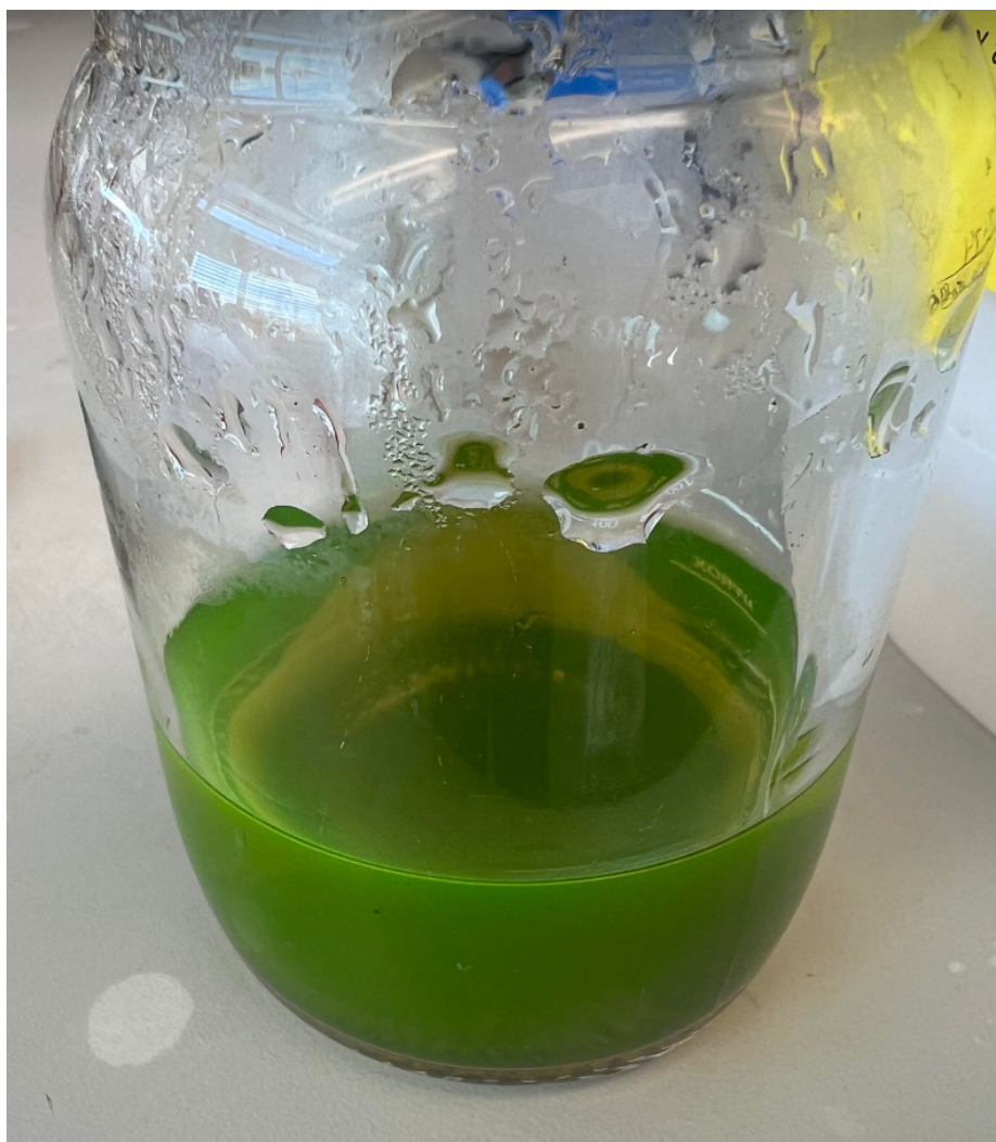
Figure F.1: The solution after using 5% copper content for recycling experiment.
