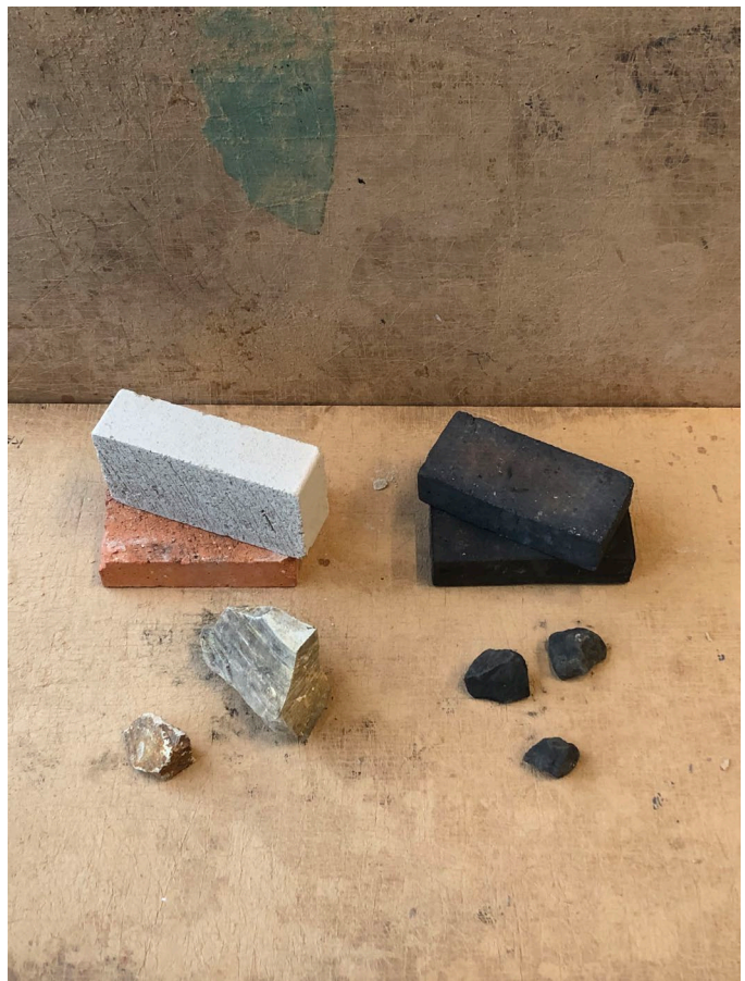
illu 84. left - colorful mo-clay and mo-clay bricks, right - ash layers and burned dark bricks
