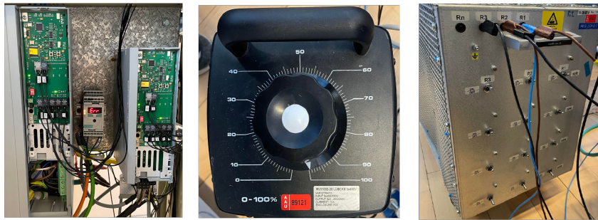
Figure 5.5: From left to right: the two inverters, the transformer and the power-resistor bank.
