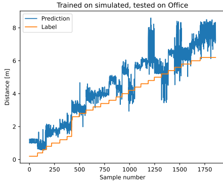
Figure 4.11: Simulation trained angle-only representation model tested on office measurements.
