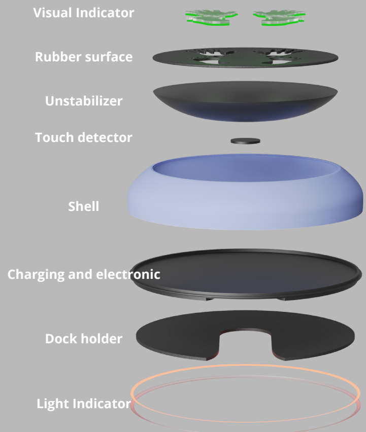
III. 85 - Exploded view phase 3
