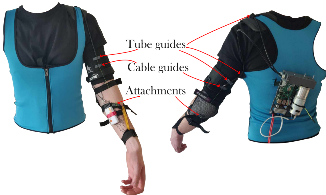
Figure 5.4: Image of the exoskeleton worn on the body from a front and back view. The cable is guided from the control box on the back to the attachment points on the forearm, through plastic guides sown into the fabric.
