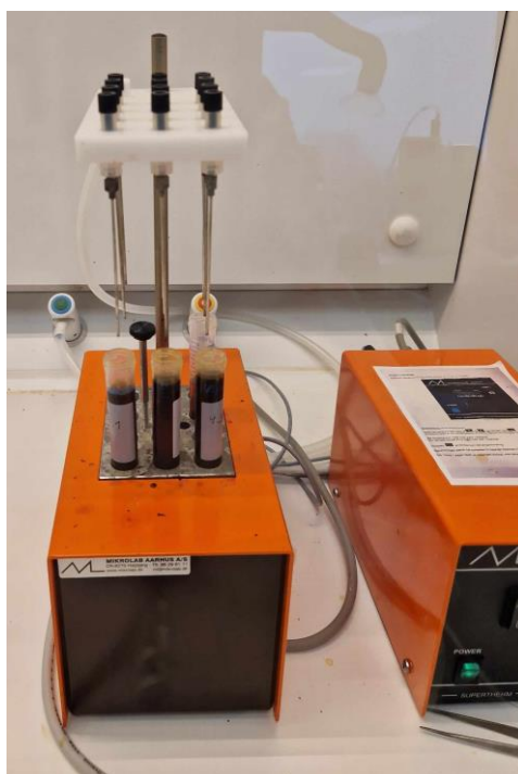
Figure 8.13: Nitrogen evaporation setup
