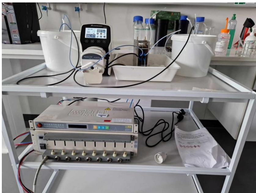
Figure 8.21: Big battery cell setup with electrolyte tanks
