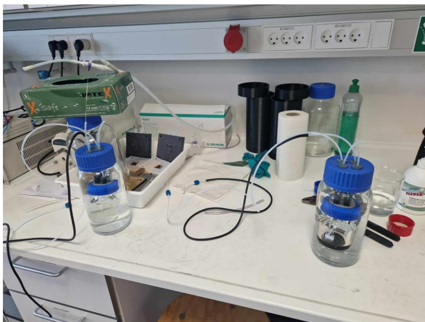
Figure 8.17: Nitrogen purging of one bottle
