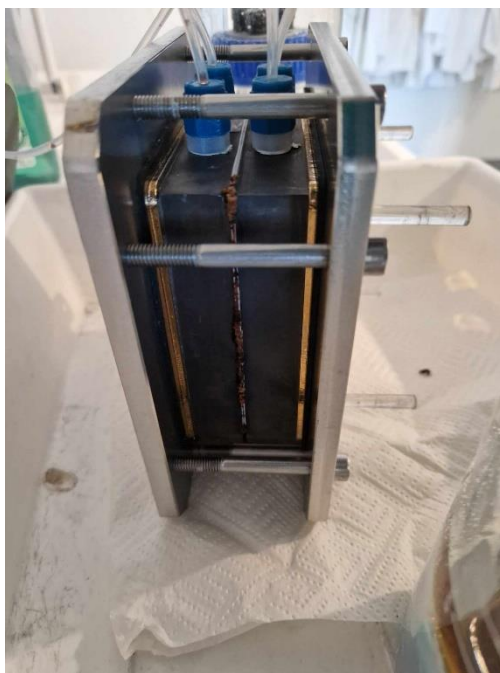
Figure 9.26: Leakage of bench-scale batch 4 battery
