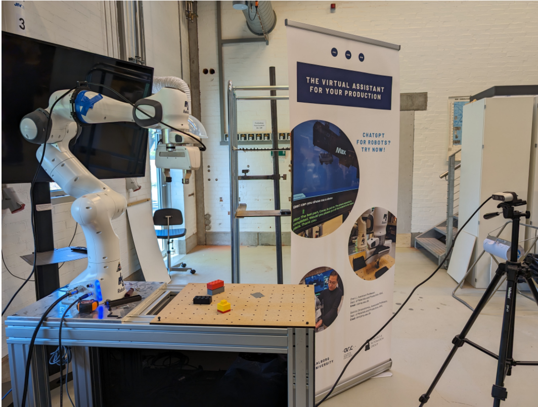
Figure 4.11: The setup of the Franka and the cameras. This position of the third person camera, is the position used for recording training data and running inference. Additionally the 4 differently colored bricks can be seen on front of the robot, with the red brick being stacked on top of the gray brick
