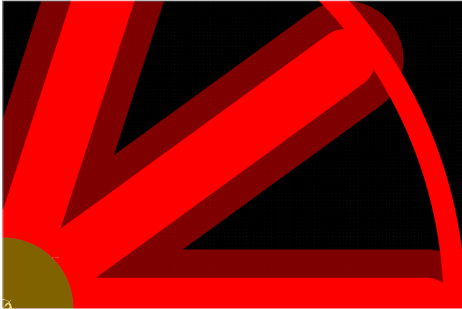
Figure 4.6: An illustration of how increasing the width decreases the possible overlap area. The figure shows two PCBs made in Altium, with one being overlaid on the other, such that a direct comparison can be made
