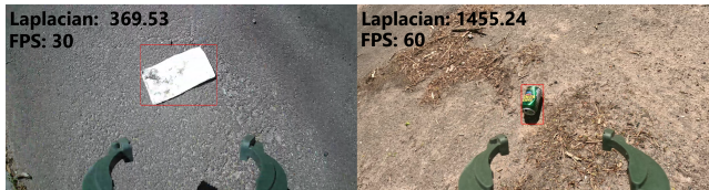
Figure 17. The laplacian of two images from the different cameras. The higher the laplacian value, the more clear the image is.
