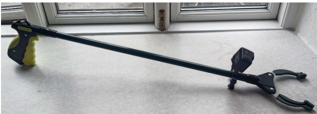
Figure 2. The litter picker with the camera mounted, ready for recording
