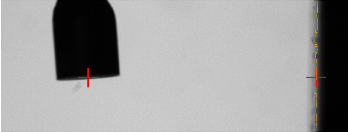
Figure 5.3: This figure shows an image of the hydrophone and the transducer used to record pressure wave data and the yellow line denotes the position the image recognition algorithm considers the transducer face. The black region along the right side of the figure is the transducer face. This figure shows the features that have been extracted from the image processing. The red '+' on the hydrophone is the calculated center of the hydrophone.
