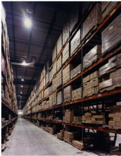
(a) Pallet racks (Storax, Inc).
