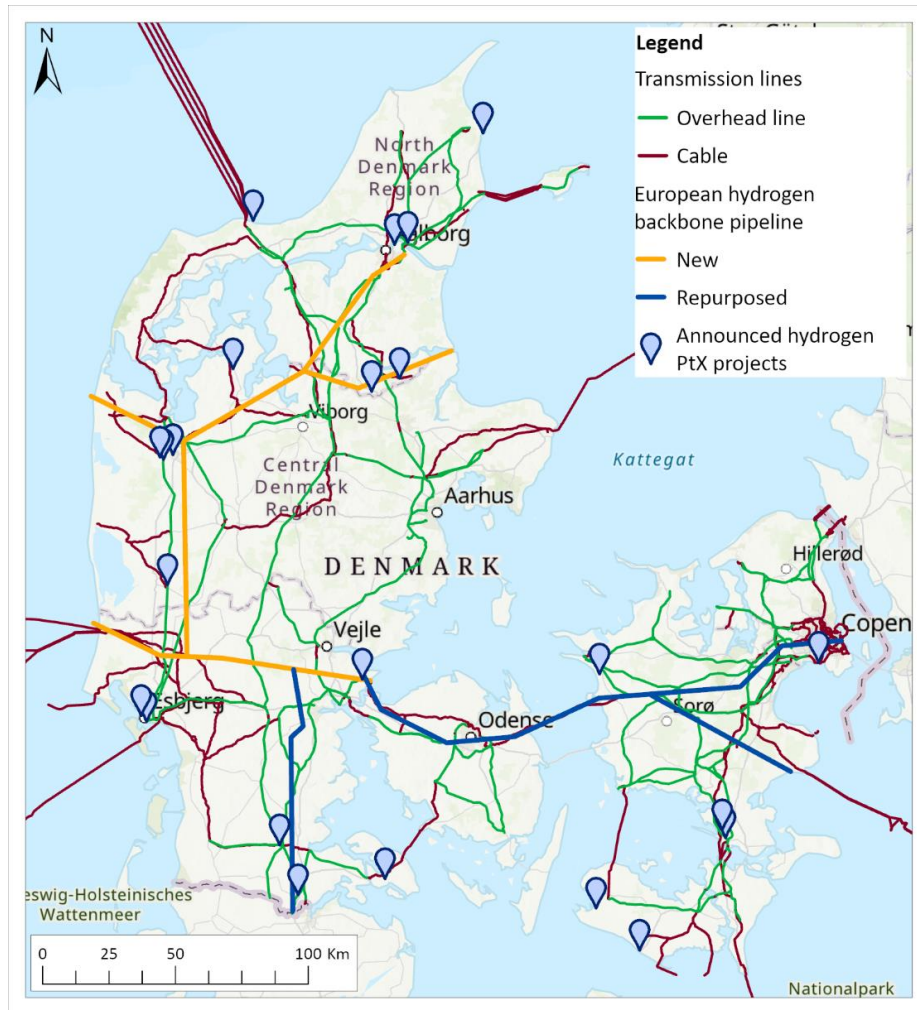
Figure 11: Proposed hydrogen pipeline, transmission lines and announced hydrogen PtX projects in Denmark [49], [81], [99], [116].
