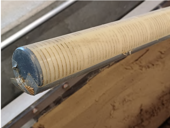
Figure 5.4: Drain pipe after conducting the experiments. Slit width of 0.8 mm and horizontal distance between the center of the slits of 0.5 cm.
