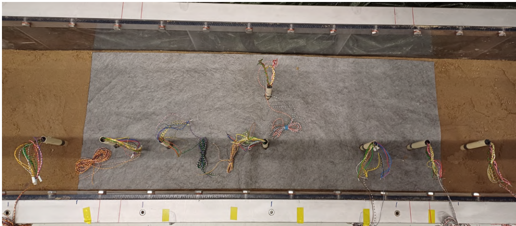
Figure 5.15: The placement of the temperature spears in the sandbox before the spears were connected. Seen from above.
