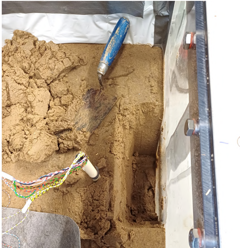
Figure 5.21: Excavation of soil behind level meter 6 (L6) to measure volumetric water content in the capillary fringe.
