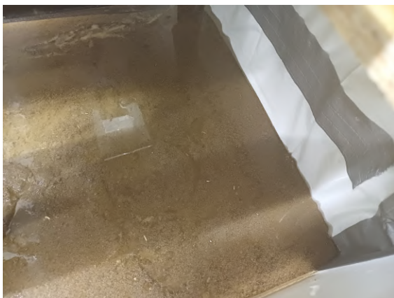
Figure 6.20: The right side of the sandbox during Warm experiment 2 seen from above. The entire surface is flooded in the right side.
