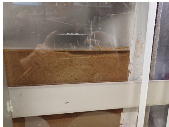
Figure 6.21: The right side of the sandbox during Warm experiment 2 seen from the front. The entire surface is flooded in the right side.
