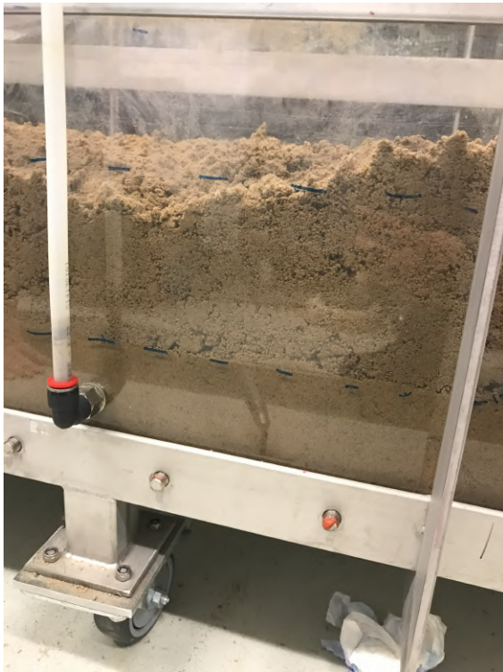
Figure 5.2: Soil layer with a compaction of 1.5 \text{ g/cm}^3 with loose soil on top.
