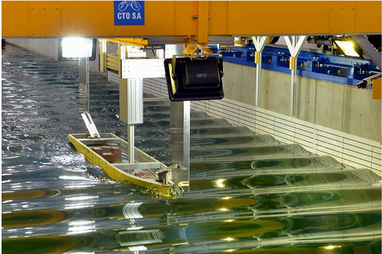
Fig 6 - Example of model test on a towing tank. Extracted from (Landowski, 2015)
