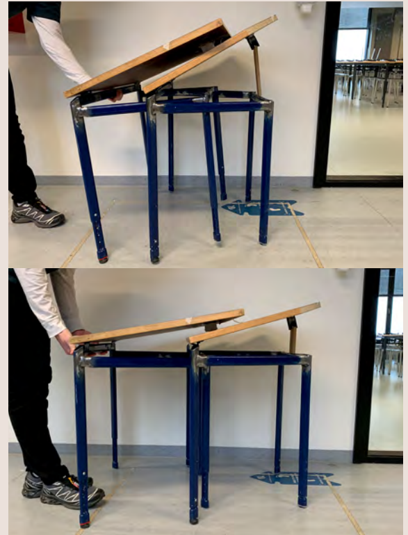
illu. 74: Test done upon stacking angle
