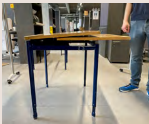
illu. 55: Test of stacking from the front
