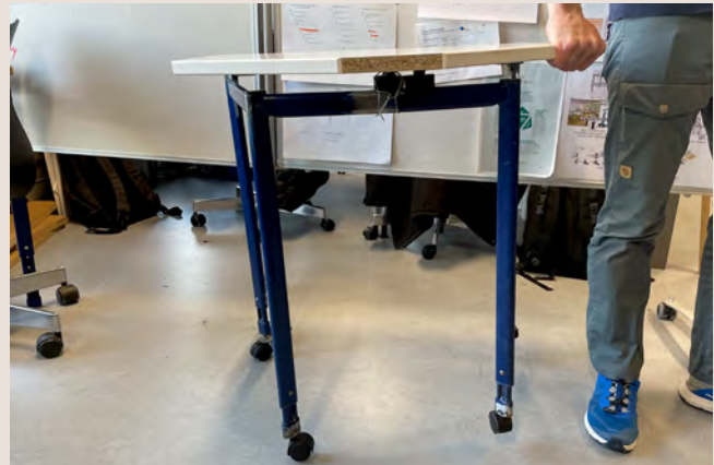
illu. 86: Stability test with one connection point
