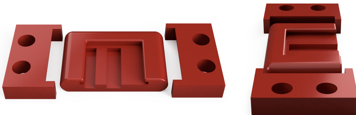
Figure 4.18. Clamping system, where microphone can be inserted into middle piece, which can then be inserted into a nitrile glove, which can then be fastened to a flat side by clamping.
