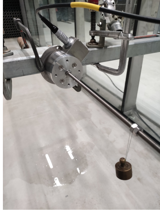
Figure B.14. Test with 200 g weight placed with an arm of 25 cm.
