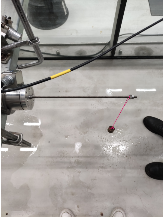
Figure B.13. Test with 100 g weight placed with an arm of 33 cm.
