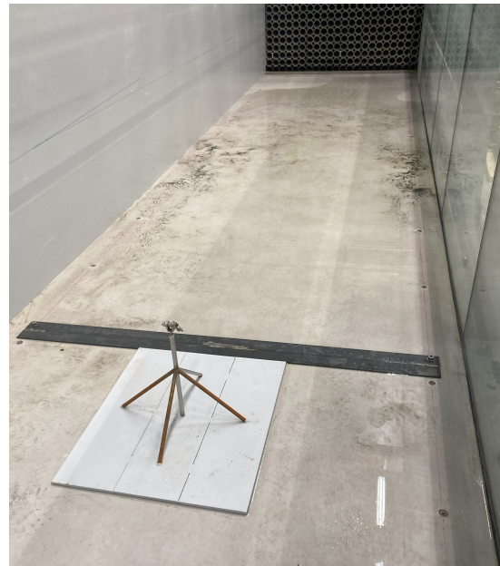
Figure 6.2. Hinge secured to the steel plate placed in the wave flume.
