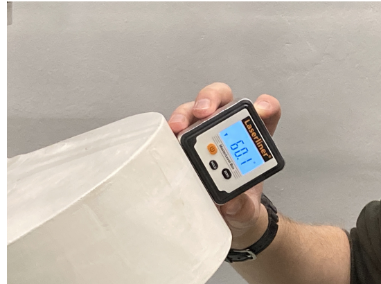
Figure B.25. The final angle of the disc at -30^\circ shown with the digital protractor.
