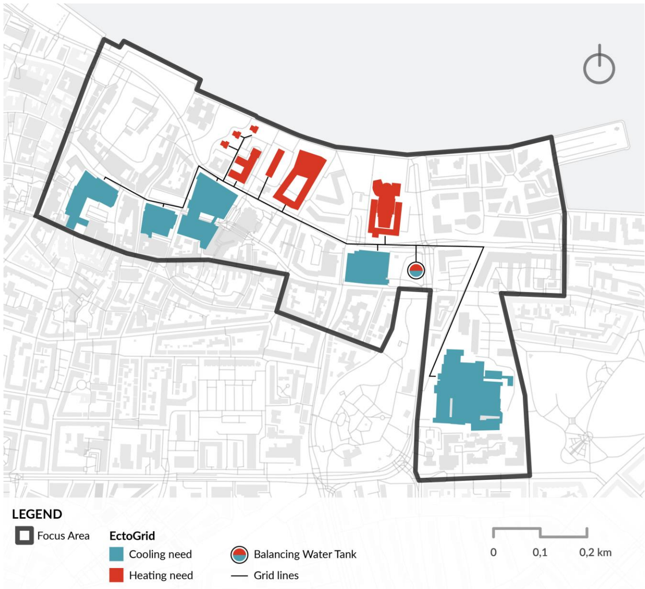
Figure 38 – Proposed installation of the Ectogrid, encompassing twelve buildings (created by the authors).
