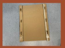
**Prototype C:** (Illustration 87) shows a concept where cutouts are made into two flanges on the cabinet allowing for hooks to enter locking the door in place.
