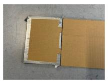
**Prototype B:** A cutout in the panel allows for two tabs mounted on the bottom of the door to attach to the back of the panel creating a seal between the parts
