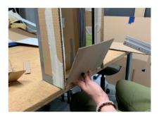
To further strengthen the attachment of the panel thread rivets (illustration 164) were inserted in the cut out previously made for the bolts. By doing so, the simplicity of the bolts were kept while enhancing the strength of the assembly.
