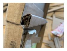
**Prototype A:** A modification of the existing solution where pressure is created when tilting the door (illustration 85) onto the 90-degree section of the panel fixing the door in place and sealing the cabinet.
