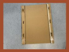
**Prototype D:** (illustration 88) is a concept where the door and panel are slid into the cabinet from the top and downwards creating a flush surface and meeting with a recess and tab that extends from side to side like prototype B.
