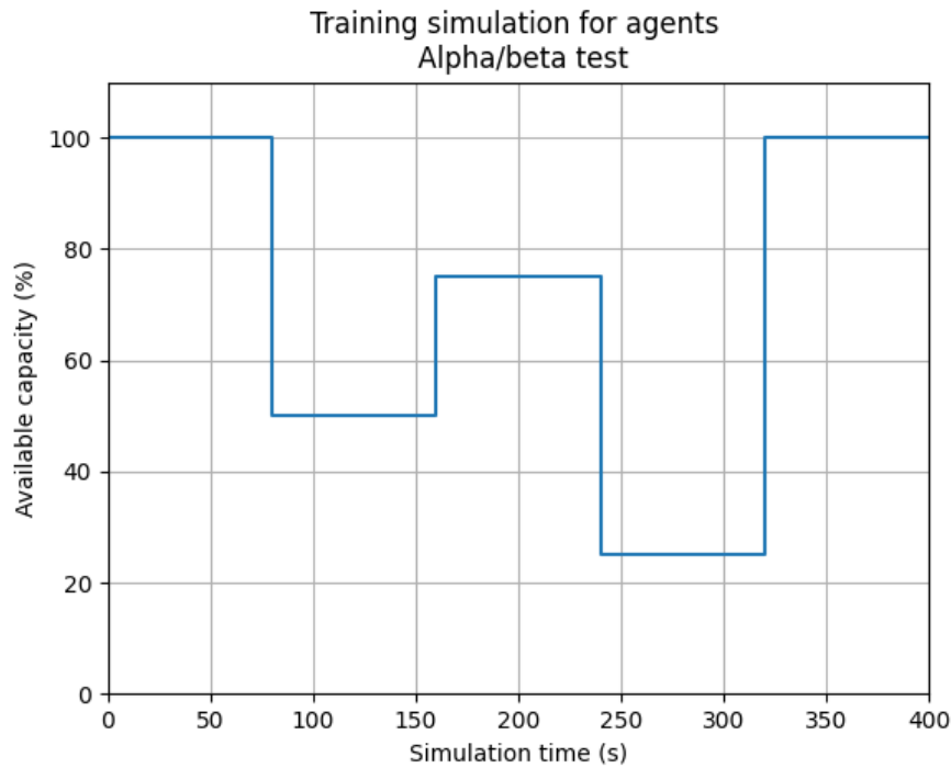
Figure 3.7. Changes in available link capacity through time during the training simulation for the alpha/beta test
