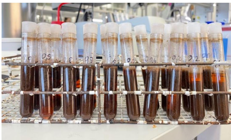
Figure 5 – 10 sample tubes filled with oil water and coagulant – EPS I + iron sulfate (pix113)
