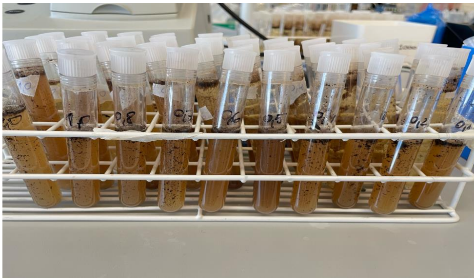
Figure 13– Picture of the samples from the second measurement (5.03) with Aragose and \text{CaCl}_2 as a coagulant
