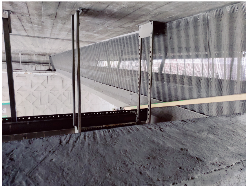
Figure 2.20. The sensor node mounted using a two by four placed over the driving lanes under the bridge
