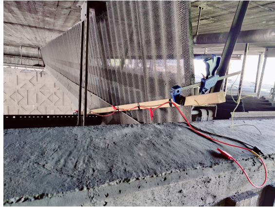
Figure 3.5. The sensor node was temporarily attached with test leads, to allow for current measurement using laboratory equipment in the real world scenario
