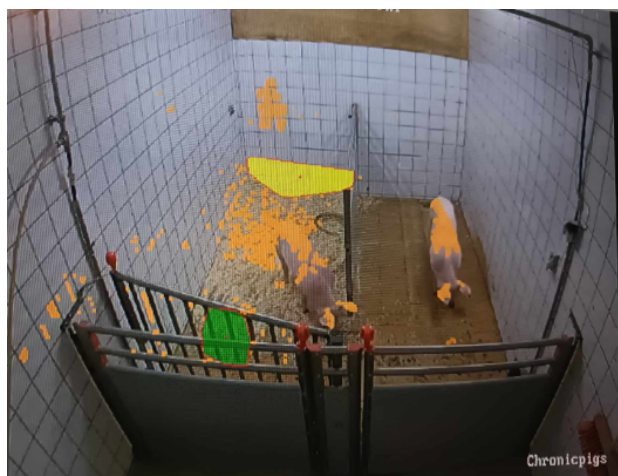
Figure C.6 Example of an incorrect tracking with a lot of noise as a result of the varying camera angles.
