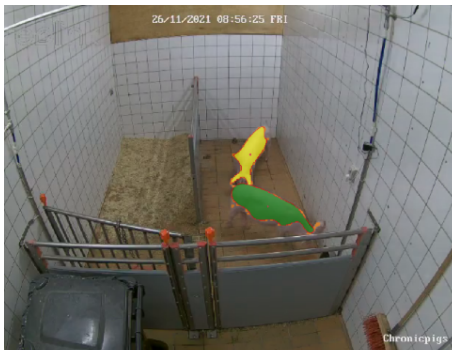
Figure C.1 Example of an image in which the contrast-based tracking using EthoVision is considered correct. The red points indicate the center of mass while the green and yellow colouring represent the tracking of the individual pigs. The orange colouring represents noise.
