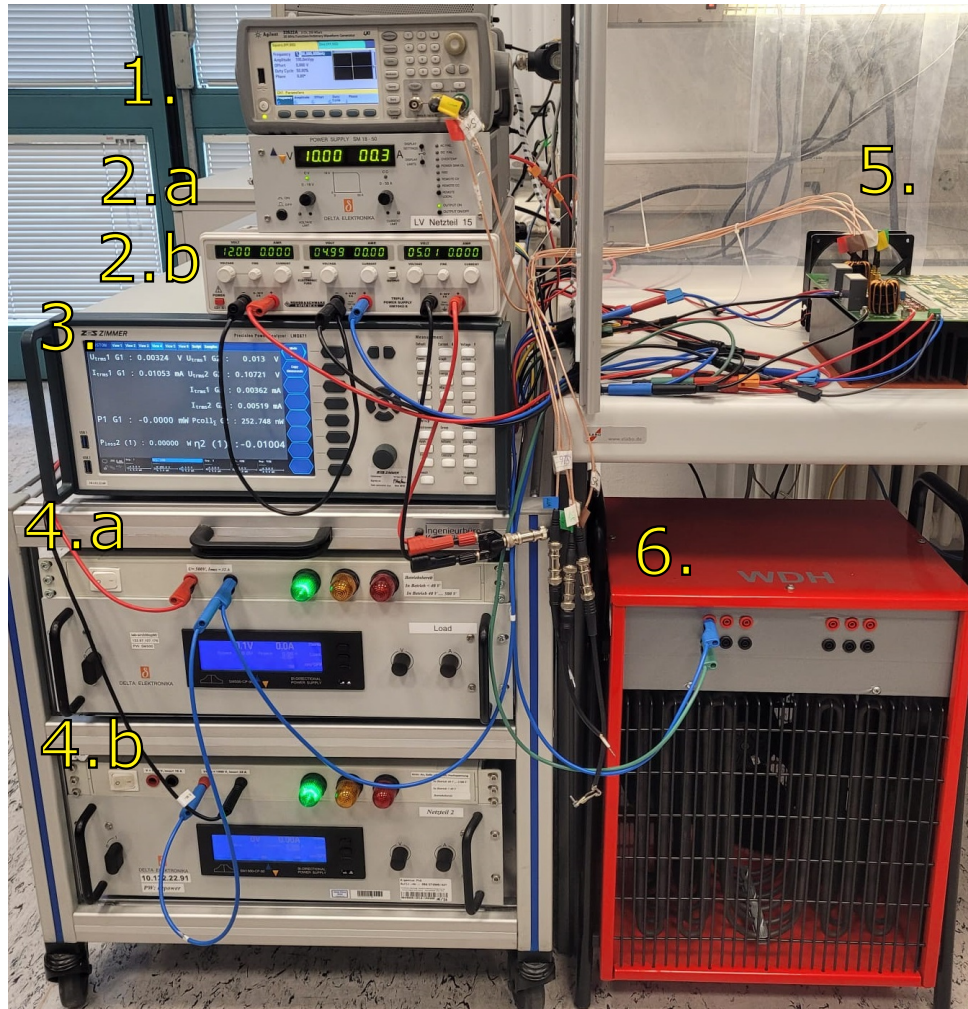
Figure 5.2: Experimental Setup. 1. PWM Generator. 2. Low Voltage Power Supplies. 3. Power Analyser. 4. High Voltage Power Supplies. 5. Device Under Test. 6. Ohmic Load.
