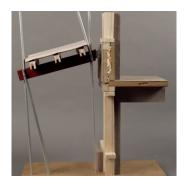
A bracket is positioned between the parapet elements and secured to the concrete column.
