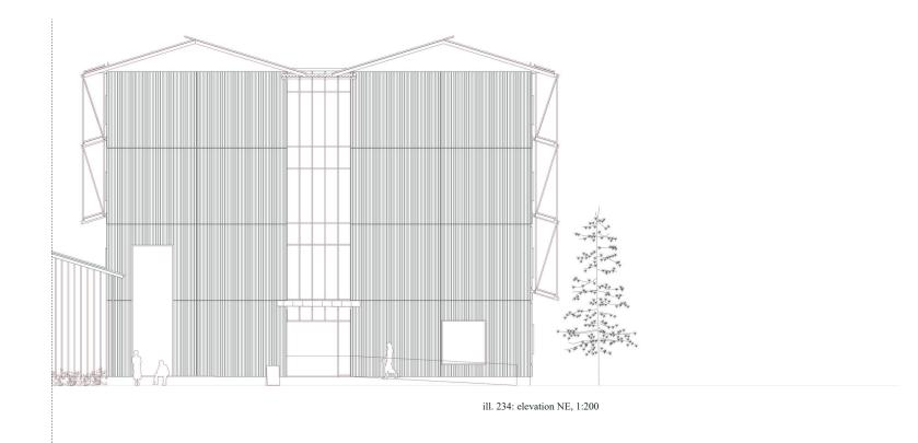
New windows are established in the gable section between the saddle roof motifs. The existing slats are removed, and vertical slats with the same center-to-center spacing as the window frames are added. This, to make maintenance/cleaning easier, to provide a greater amount of light indoors, and to improve the viewing opportunities. The depth of these slats is still perceived in the same rhythm and density when viewed from the street, due to an increased depth.
