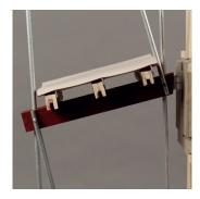
Under the asbestos-cement roof, three painted wood battens are placed at 1000 mm intervals.
