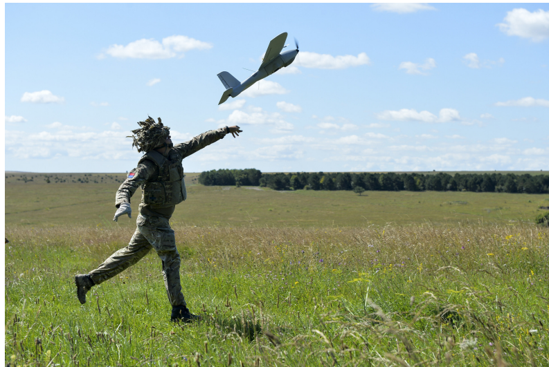
Figure 2.1. Launching of a Desert Hawk III [10]
