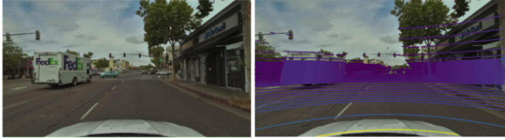
Figure 3.8. Lyft L5 dataset Example from ego vehicle, Left: original image without labels Right: The image and point cloud data collected. [17]
