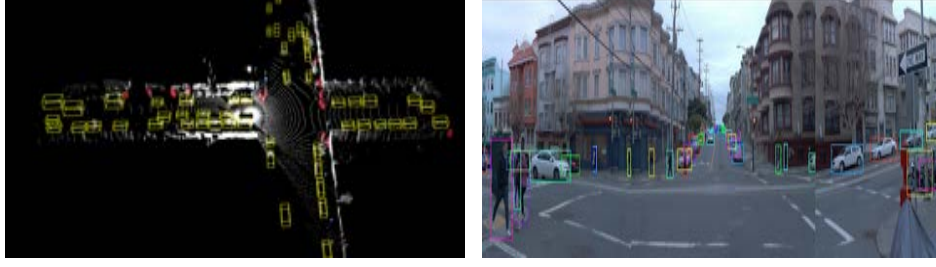
Figure 3.10. Waymo Example from ego vehicle, Left: Birds-eye-view LiDAR image with labeled ground truth 3D bounding boxes Right: View from front, front left and front right cameras with the labeled ground truth 2D bounding boxes. [20]
