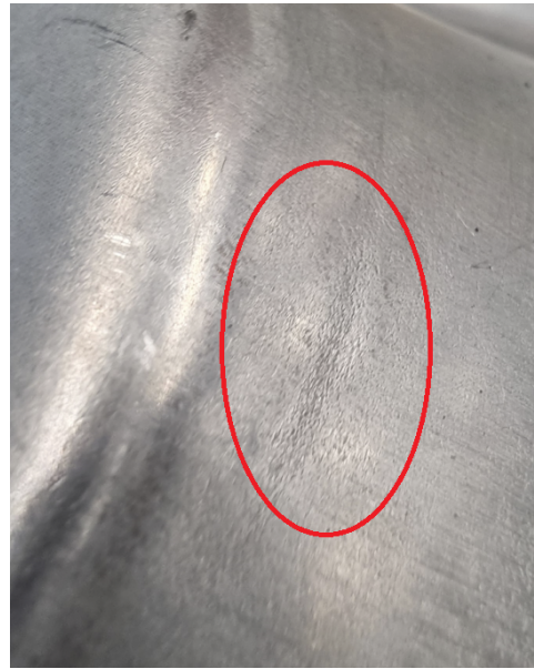
(b) Severe material stretching.
