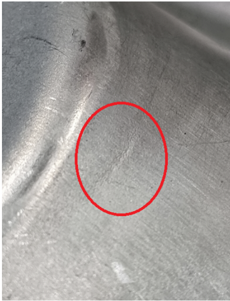
(a) Minor material stretching defect.
