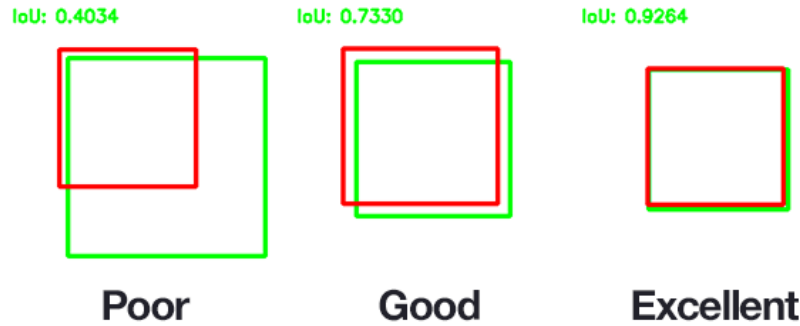
Figure 3.3: An image illustration how IoU may be interpreted. Source: By Adrian Rosebrock - http://www.pyimagesearch.com/2016/11/07/intersection-over-union-iou-for-object-detection/ , CC BY-SA 4.0, https://commons.wikimedia.org/w/index.php?curid=57718559
