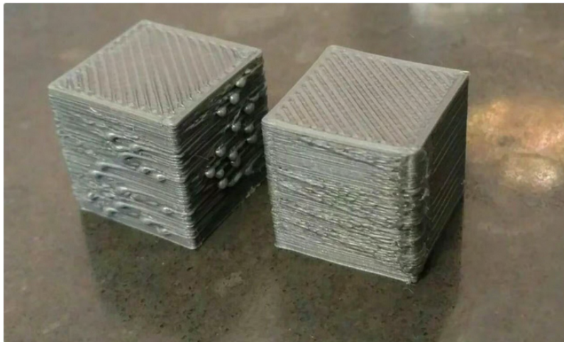
Figure 2.11: Printed objects having blobs and zits on the walls [5]
