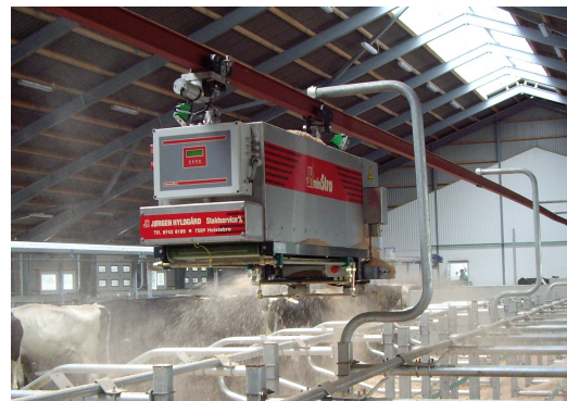
Picture 2: Littering robot
