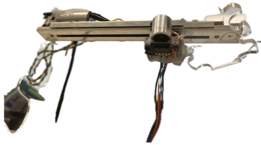
Figur 3.4: The distance sensor and laser mounted on the fader.
