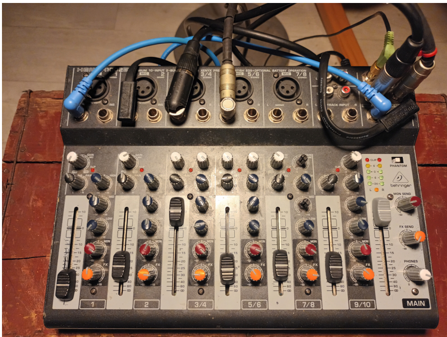
Figure 3.1.: A simple no-input mixer setup: channel 1 is in feedback through the AUX send, channel 2 through the FX send, channel 3 and 4 get the main outputs, while sound is sent to speakers from the headphones out. These feedback connections are embedded at the circuit level on our mixer.
