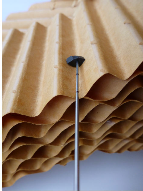
Figure 4.14: The scraper scraping a clean Muntz filter of type D. The two marked black lines on the scraper indicate 1 cm each. The black rubber on the scraper is 1.1 cm in width.
