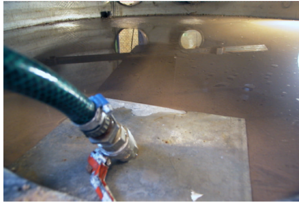
Figure B.5: Hose connected to plate which is used to fill the tank with water after the sand is vibrated and leveled.
